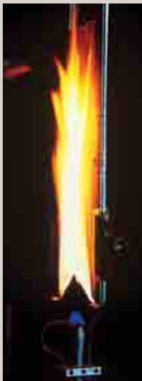
Vertical flame test on non-flame resistant fabric
